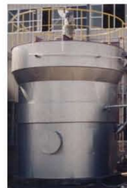
Aluminum hydroxide-separation crystallizer
