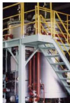
Glauber's salt-separation crystallizer
