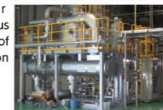
Ejector FFC Type Plating-related Effluent Concentrator
